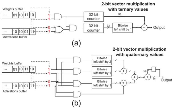
Figure 4: This figure illustrates the hardware implementation of the dot product between, (a) ternary weights and ternary activation (b) 2-bit weights and 2-bit activation.
