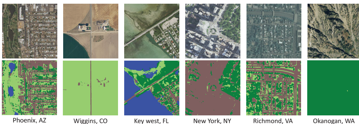
Figure 1: National Agriculture Imagery Program (NAIP) aerial imagery ( top row ) with modeled land cover estimates ( bottom row ). Existing supervised learning models, trained for generating land cover labels from aerial imagery, do not generalize well due to the large spatial and temporal variances in aerial imagery. Creating accurate land cover maps at a massive scale therefore requires additional human interventions. We propose an interactive model fine-tuning system, coupling human labelers and machine learning models, for facilitating these interventions.
