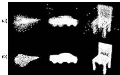
Figure 8: Projected predictions trained (a) without and (b) with affinity loss, which helps in outlier point removal.
