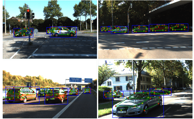
Figure 1: Representative 3D detection results, shown as projections on the input images. 3D morphable shape models of each vehicle are colored in green. Dashed green lines are occluded edges. For the 14 vertices of each morphable shape model, visible vertices are colored in red and occluded ones in yellow. 2D bounding boxes are colored in blue.
