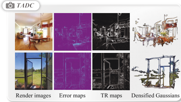
Figure 5: Error maps show the intensity of inconsistency between the rendered image and the ground truth. We observe that Regions with high texture richness are often under-optimized. Therefore, we propose TADC dynamically control the density of Gaussians according to texture richness.
