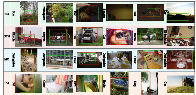
Figure 6: Sample detection results. Red boxes represent the ground-truth annotation. Green boxes indicate correct detection results. “BG” represents samples that are easily confused with the background. “OTH” indicates samples that are easily confused with other categories. “MC” shows samples that are located in messy surroundings. “PO” denotes samples that are shown partially.
