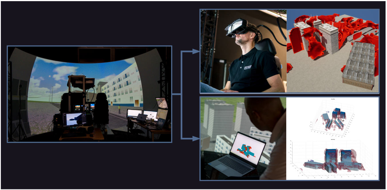
Figure 2: Full flight simulator architecture and visualization pipeline. The Level D H145 simulator provides six degrees of freedom motion, high-fidelity out-the-window (OTW) visuals, and a fully replicated cockpit. Hazardous wind regions are depicted as volumetric geofences, rendered in real time via OTW and optional VR (Unreal Engine 5). The pilot’s headset visualization supports operational awareness and avoidance of critical areas. Aircraft state is received via UDP; hazard volumes are derived from wind-field features, encoded as STL, and streamed for display, furnishing the pilot with an additional source of turbulence information.
