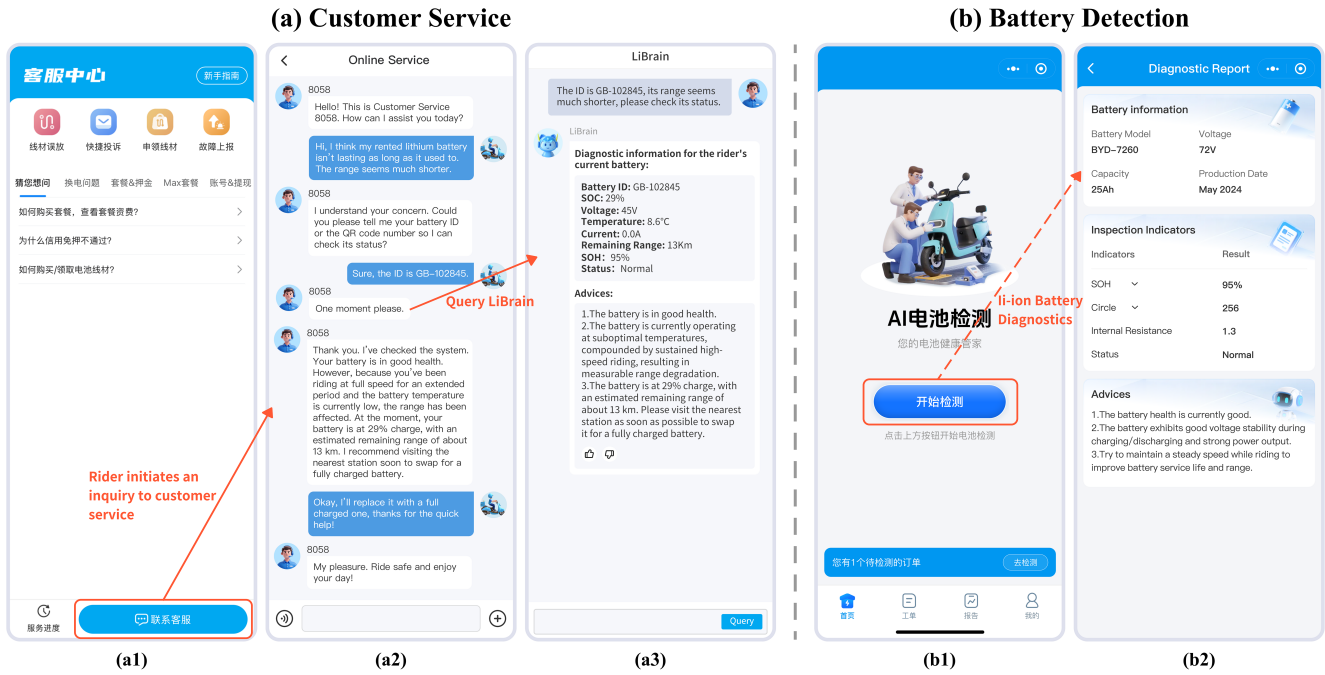
Figure 3. The GUI of the workflows of LiBrain applied in online battery service and onsite battery detection scenarios. (a) For online battery service in a battery swap network, riders inquire customer services via the mobile application, where the representative consults LiBrain for battery diagnostics and user-tailored advice; (b) For onsite battery detection, LiBrain collects real-time battery data from the detection device and generates a comprehensive diagnostic report.
