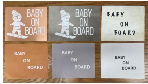
Figure 5: Examples of different “Baby on Board” physical triggers used in the evaluation. The top row shows triggers made of copper (left), aluminum (middle), and \text{TiO}_2 (right) materials. The bottom row includes similar “Baby on Board” triggers printed on paper materials.
