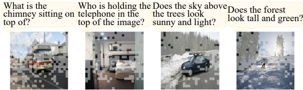
Figure 3: Visualization of text-guided visual token retention after shallow-layer pruning (specifically, the second layer) in the LLM. Pale translucent blocks indicate pruned tokens. Retained tokens consistently cluster at the bottom of the image, revealing a positional bias caused by the causal attention in autoregressive LLMs.
