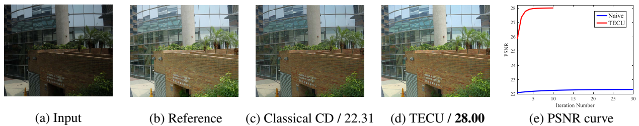
Figure 2: Comparisons between the classical CD algorithm, i.e., PAM (Attouch et al. 2010) and TECU. The PSNR scores are reported below (c) and (d) sub-figures. The PSNR curves with respect to iteration number is plotted in sub-figure (e).
