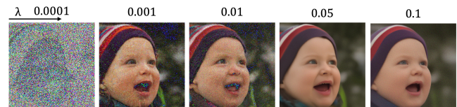
Figure 7. Effect of hyperparameters \lambda . Reconstructed images from the same 1-bit CS measurement with input images corrupted by additive Gaussian noise of \sigma = 0.5 .
