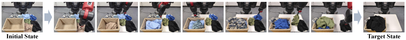
Figure 6: Real-World Robotic Cluttered Cloth Storage. For the cluttered cloth piled on the table, our framework can accurately perceive the area of each piece of cloth and estimate the corresponding wrinkle position that is easy to grasp. The robot places each piece of cloth on the table into the storage basket sequentially according to the obtained grasping position sequence, confirming the real-world effectiveness of our method.
