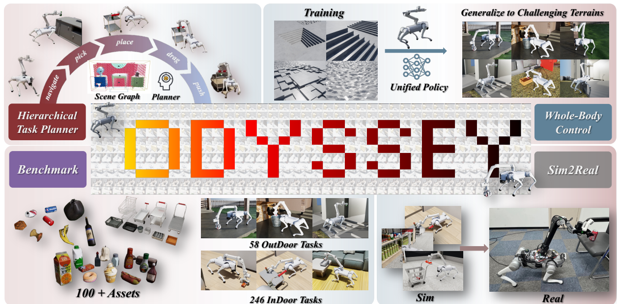
Figure 1: We present ODYSSEY, a unified mobile manipulation framework for agile quadruped robots equipped with manipulators, which seamlessly integrate high-level tasks planning with low-level whole-body control.
