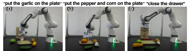
Figure 4: Real robot manipulation tasks used for physical validation of TTF: (a) single-object pick-and-place, (b) multi-object sequential manipulation, and (c) contact-rich drawer closing.
