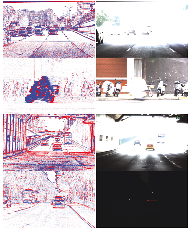
Figure 1: PEOD examples under diverse challenging conditions. Overexposure (rows 1-3), motion blur (row 2), and low-light (row 4). Each row presents the event stream (left) with its pixel-aligned RGB frame (right).
