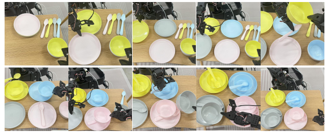
Figure 3: Real-world deployment: Two XLeRobot manipulators collaboratively completing a tableware setting task using PIPHEN. By sharing compact physical semantics ( \sim 5\% data volume) rather than high-dimensional video streams, PIPHEN enables precise, smooth multi-step collaboration, effectively addressing the “shared brain dilemma” in physical interactions.
