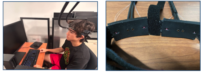
Figure 2: Setup: Participants sat 24 inches in front of a computer screen. The fNIRS device is a headband that shines pulsating infrared light into the PFC to detect changes in blood flow.
