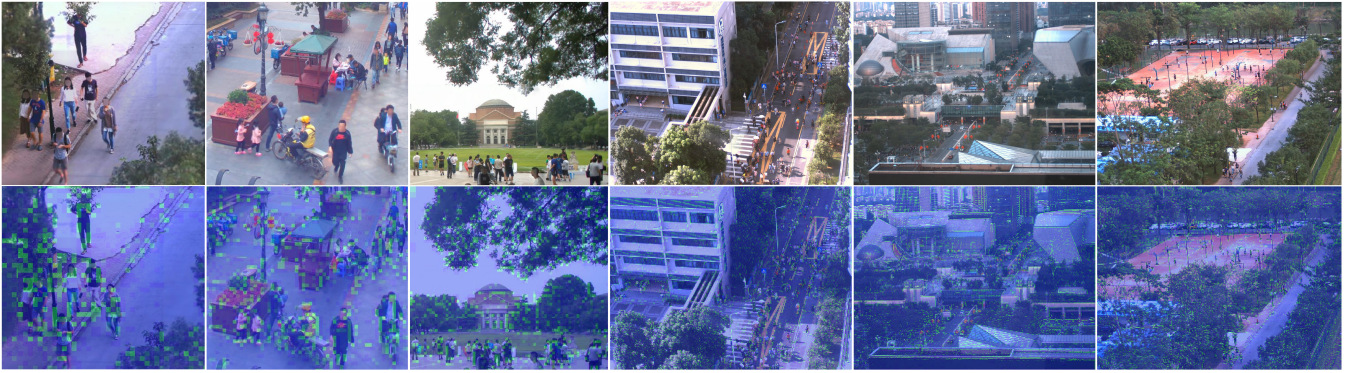
Figure 3: Visualization of first-stage expert allocation for GigaMoE on the PANDA dataset. The original images (top) are shown with their corresponding expert allocation maps overlaid (bottom), where warmer colors (from blue to green) signify a higher computational budget. GigaMoE intelligently allocates computational resources to complex regions, such as dense crowds, vehicles, and richly-textured foliage. It also focuses on object edges, including building facades, road curbs, and traffic markings. In contrast, semantically simple areas like the sky and open ground receive minimal resources (deep blue).
