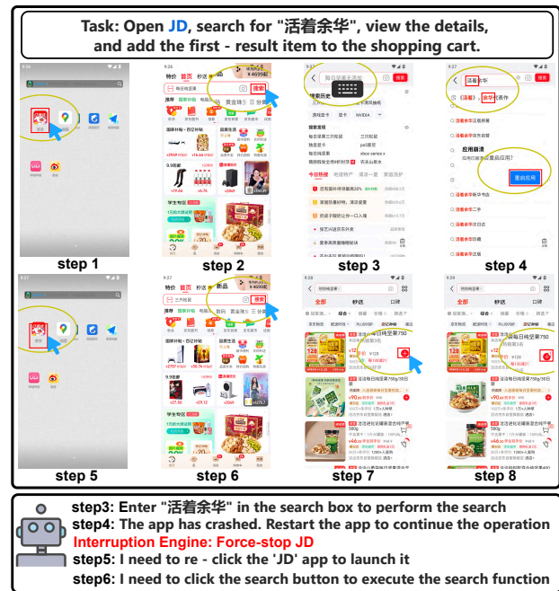
Figure 4: A case of perceptual drift after App crash recovery. The black and red dash indicate normal and interruption path, respectively.
