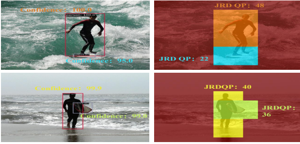
Figure 2: Relationship between the confidence score and the object region JRD level ( i.e. , coding unit-level QPs).
