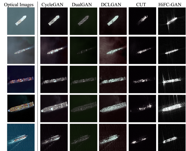
Figure 3: Comparison of intermediate domain generation results on the Optical-to-SAR task. We compare HiFC-GAN with existing methods and HiFC-GAN shows visually satisfactory results. The first column shows the input to the generator.
