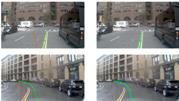
Figure 4: Visualization results across various challenging scenarios. In each example, the green trajectory represents the ground truth from the human expert, the red trajectory is generated by Hydra-MDP++, and the blue trajectory is produced by DriveSuprim.
