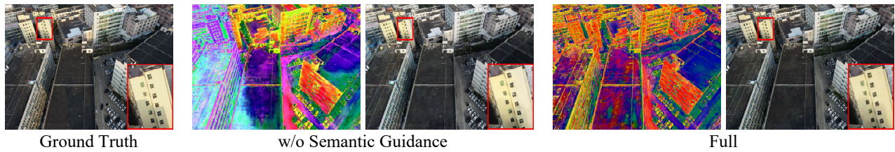
Figure 4: Visualization of the effect of semantic guidance in CAG-GS. Anchor feature maps and rendered RGB images of CAG-GS with and without semantic guidance are shown, along with the ground truth RGB image. The current view covers two blocks, and the color shift in the first feature map marks their boundary.
