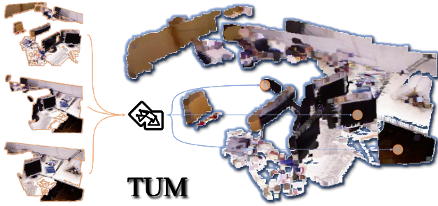
Figure 3: GICP Mismatches in TUM Scenes. Even with high-precision depth data, real-world noise can lead to misalignments in GICP-based pose estimation, as illustrated here in the TUM dataset.
