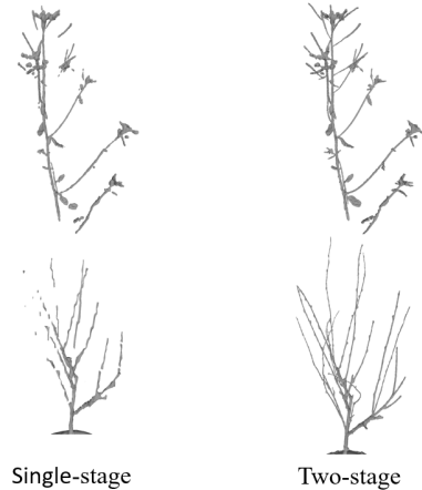
Figure 5: Comparison of final reconstructed meshes. (a) Using single-stage masks without geometric priors results in background noise and missing structures. (b) Using our two-stage mask extraction with geometric priors improves foreground completeness and detail, confirming the benefit of geometric guidance.
