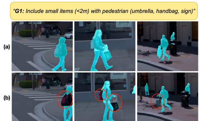
Figure 2: Annotation inconsistencies in the Waymo segmentation dataset. Row (a) shows masks adhere to guideline G1 at timestamp t , while row (b), from the same scene at t + \Delta t , shows a clear violation of the same guideline.
