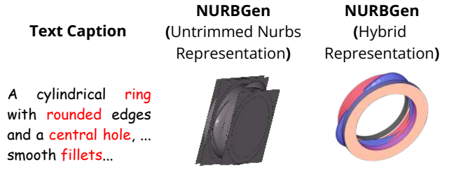
Figure 8: Comparison of NURBS-only (left) and hybrid (right) models, showing improved handling of thin and hole-adjacent regions.
