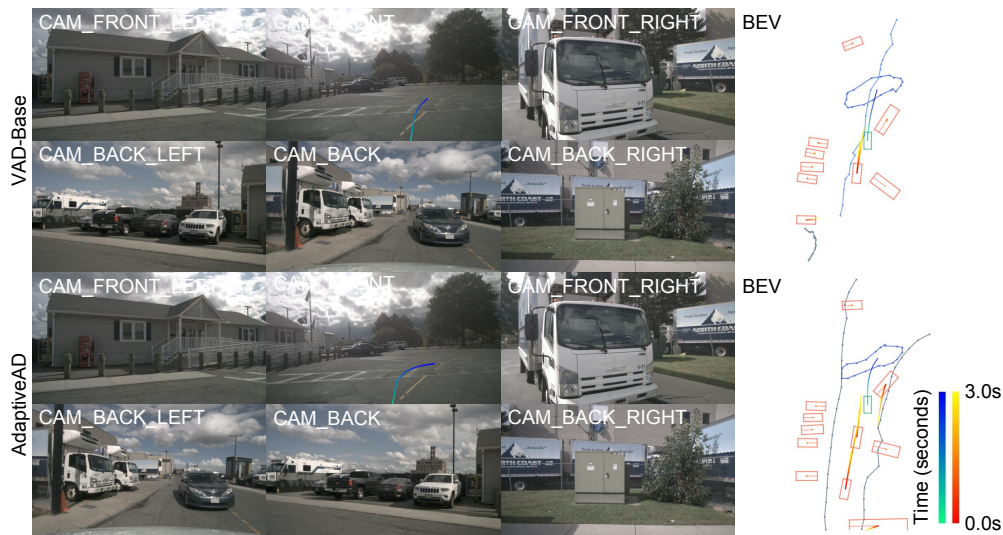
Figure 5: Qualitative comparison of scene generalization ability. In this challenging scenario, our AdaptiveAD demonstrates significantly superior perception capabilities compared to VAD, providing more reliable obstacle-avoidance paths.
