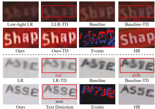
Figure 1: Examples of EvTSR. We illustrate two major challenges in TSR: poor lighting and motion blur. Both hinder accurate text localization in LR images and degrade recognition. Existing TSR methods struggle with these issues. By incorporating event cameras and our proposed EvTSR approach, text clarity and localization are significantly improved. (TD: text detection; HR: high-resolution)
