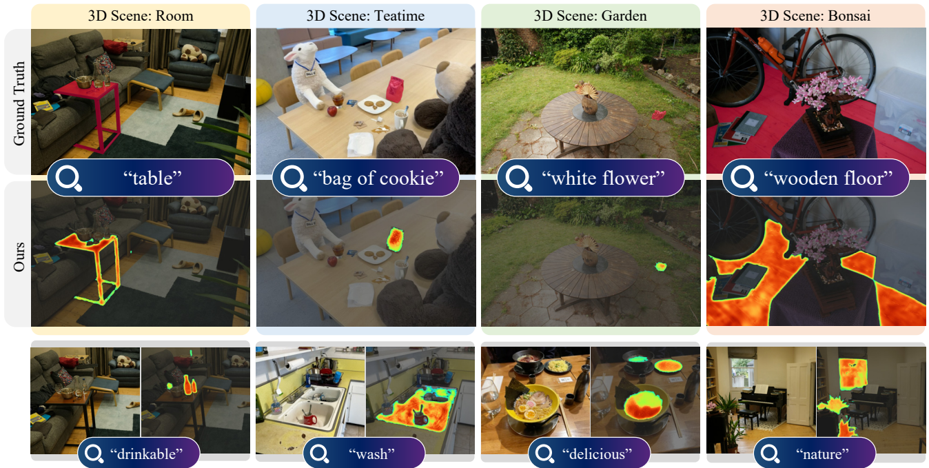
Figure 2: Given multiview images of a scene, GAGS learns a 3D Gaussian field associated with semantic features, which enables accurate open-vocabulary 3D visual grounding in the scene.
