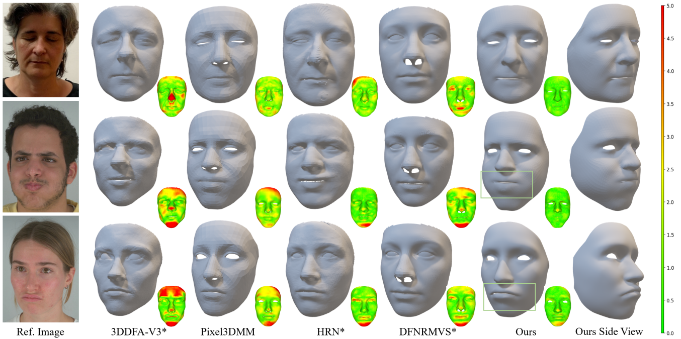
Figure 3: Qualitative comparison on the H3DS benchmark (the first row) and the NeRSemble benchmark (the last two rows). For each result, we pair it with the error map against the GT scan. Methods marked with * adopt the BFM topology with around 40000 vertices, while Ours and Pixel3DMM follow the FLAME topology with around 5000 and 1500 vertices, respectively.
