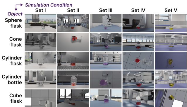
Figure 1: Simulation samples of five transparent containers under five distinct simulation sets from Phys-Liquid, showing variations in laboratory scenes, lighting conditions, container rotations, liquid colors, volumes, and deformations.
