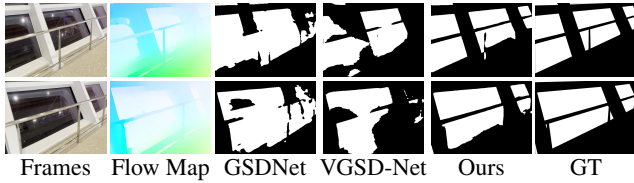
Figure 2: Existing methods may under/over-detect glass surfaces in challenge scenes. Our method utilizes motion inconsistency cues to guide GSD and outperforms competitors.
