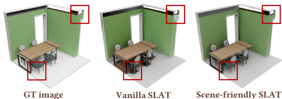
Figure 3: Scene-friendly SLAT better models 3D scene blocks, particularly in areas with occlusions and near block boundaries.
