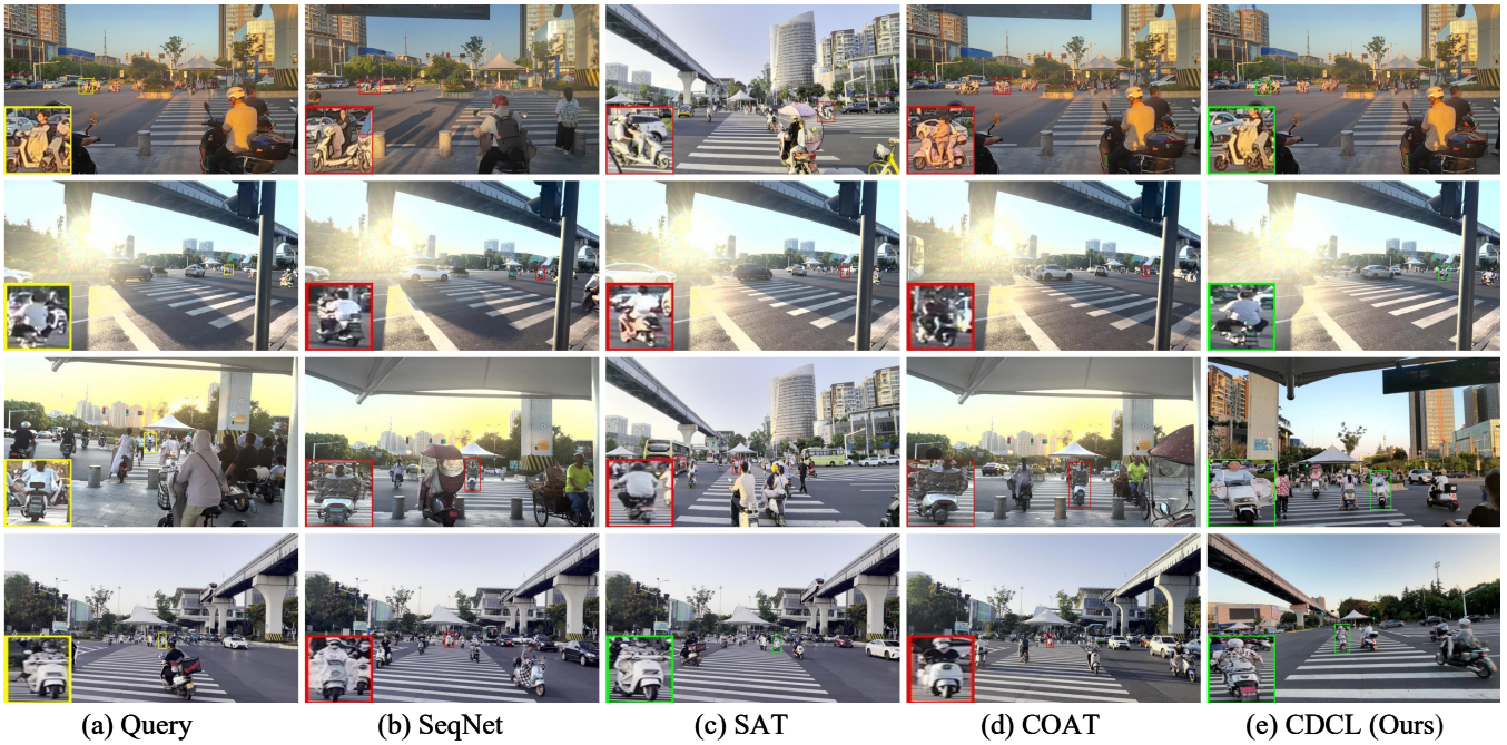
Figure 5: Qualitative comparison of our CDCL with SeqNet, SAT and COAT methods on the EBRS dataset. The yellow bounding boxes denote the queries, while the red and green bounding boxes indicate incorrect and correct top-1 matches, respectively.
