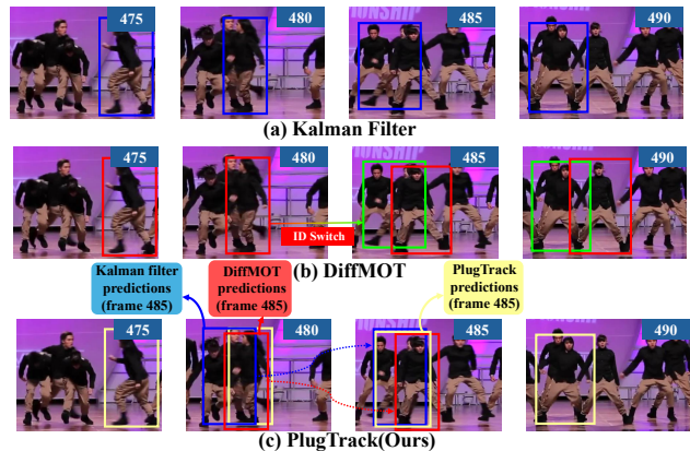
Figure 4: Qualitative comparison on DanceTrack dataset showing tracking results across frames 475-490. (a) Kalman filter maintains ID consistency. (b) DiffMOT suffers from ID switching at frame 485. (c) PlugTrack (Ours) successfully maintains ID consistency through adaptive blending ( \alpha_x=0.874 , \alpha_y=0.413 ) Boxes of the same color indicate the same tracked identity.
