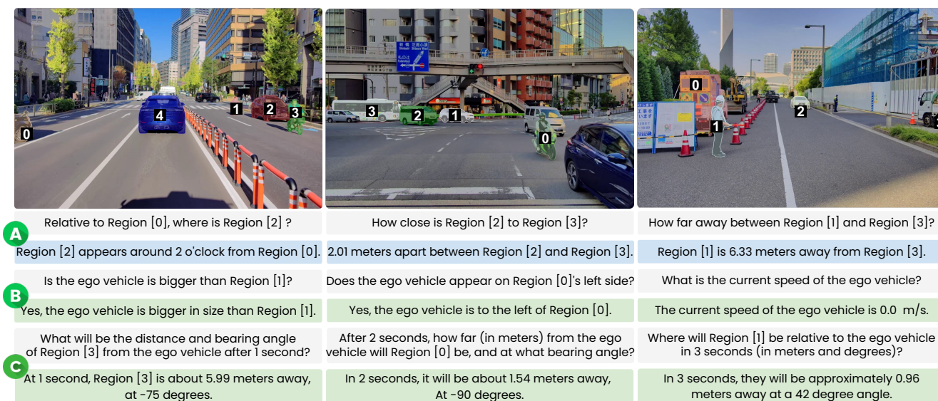
Figure 2: Example data from our STRIDE-QA dataset. From top to bottom, each QA pair corresponds to (A) Object-centric Spatial QA, (B) Ego-centric Spatial QA, and (C) Ego-centric Spatiotemporal QA.
