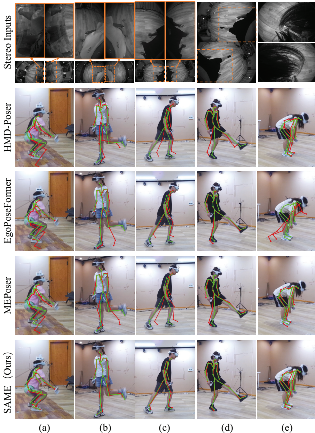
Figure 5: Qualitative comparison on a few challenging inputs. For better illustration, the predicted (red) and ground-truth (green) 3D poses are re-projected onto external reference views which are not used for pose estimation. Note that the input IMU data is not presented in this figure for simplicity. The qualitative results confirm that our SAME obtains more accurate 3D poses than existing single-modal and multi-modal methods. Best viewed in color.
