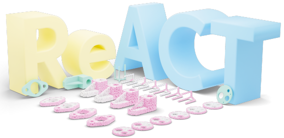
Figure 1: CAD models (green), their full surface point clouds (white), and scaffolds (pink) formed by the cumulative LBPs extracted after each sketch loop closure. These scaffolds capture extrusion sidewalls and sketch contours, providing progressive structural context for ReACT 's scaffold-aware geometric attention.
