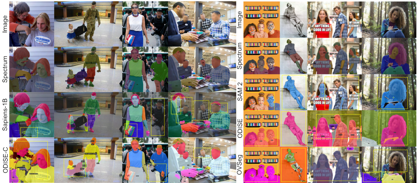
Figure 6: (Left) Multihuman Grand-f: ours surpasses Sapiens-1B and retained ODISE-C. (Right) Open-vocabulary parsing in the wild: baselines merge all people into one mask, whereas ours preserves distinct clothing and body-part masks.
