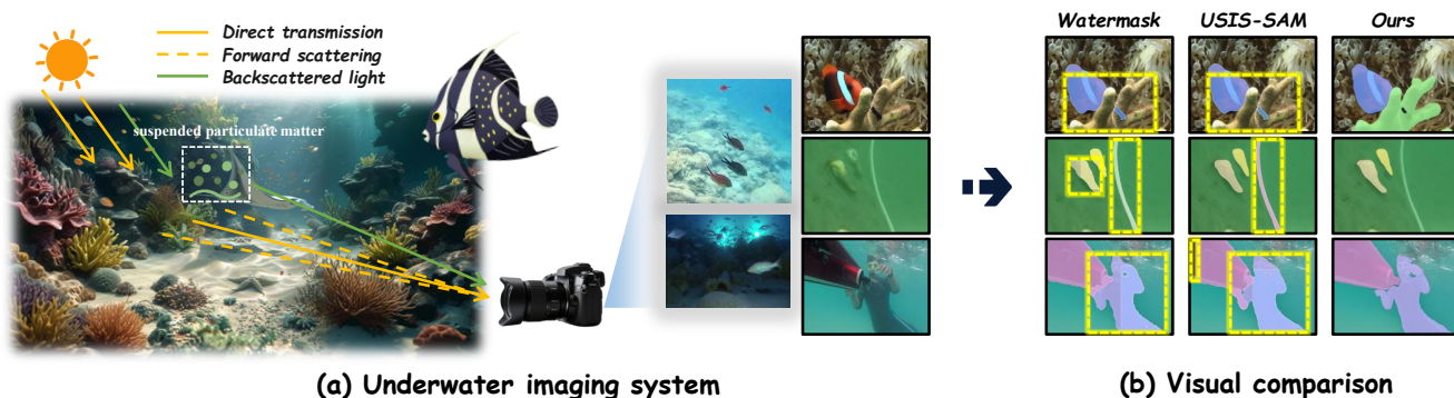
Figure 1: (a) A typical underwater imaging system: direct transmission carries useful scene information, forward scattering causes blurring, and backscattered light reduces visibility. We also present representative underwater images from UIS datasets. (b) Visual comparisons among Watermask (CNN-based method), USIS-SAM (SAM-based method), and Ours (DINO-based method).
