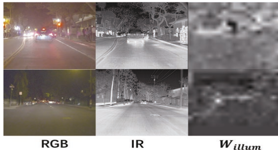
Figure 6: Visualizing the illumination weight in Equation 4 reveals that different weights are dynamically assigned to different lighting conditions.
