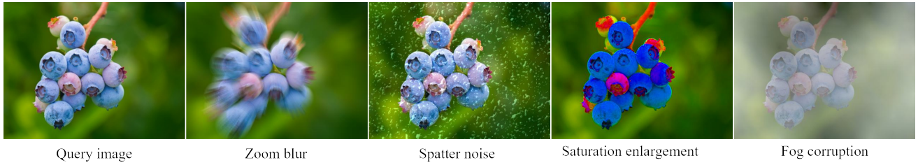
Figure 3. Illustration of the four distortion types which could degrade image quality significantly while largely preserving its semantics.
