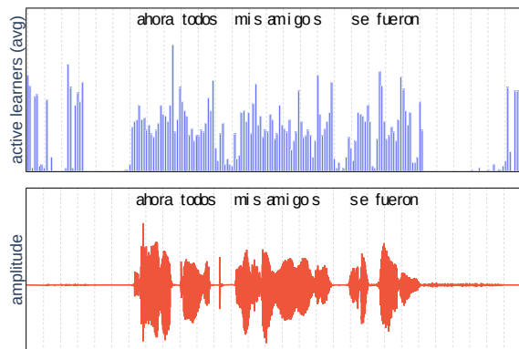
Figure 7: For each input audio token (red waveforms), we show the average number of learners that were activated in the ACMized model for \beta_{\text{target}} = 0.25 (blue bars). We can see that this model also learned to allocate its computational budget to important regions of the input.
