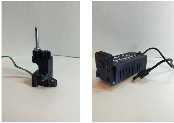
Figure 3: Left : The motor used to rotate the cleaning blade in our example desk cleaning robot (see Fig. 2). Right : Robot MCU and integrated camera
