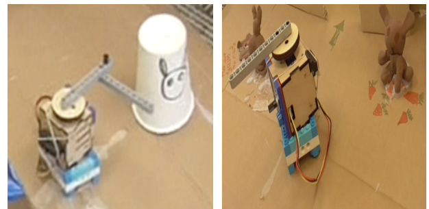
Figure 6: Group 1 used a Smart Motor and distance sensor to hit rabbits for the Novel Engineering-inspired activity in session 3.
