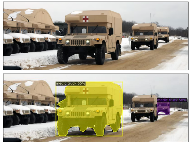
Figure 1: Example of a nuanced class, where the medic truck is only slightly different from the regular truck. Top : Original image with two medic trucks interspersed with non-medic trucks. Bottom : Demonstration of our system correctly detecting only the two desired medic trucks.
