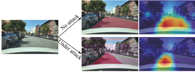
Figure 6: Model attention variations across attack intensities in the case of “drivable area reduction”.
