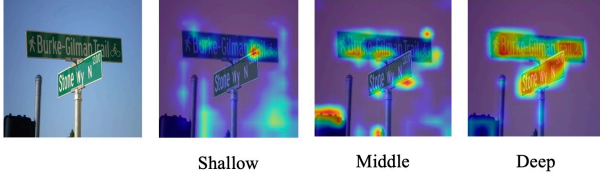
Figure 5: Visualization of MAE’s features. The model captures low-level information in shallow layers and shifts focus to semantic parts as the network deepens.
